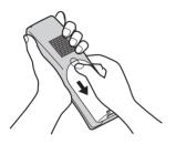
2 Insert the battery (●), and press it down until it snaps into position (②).
